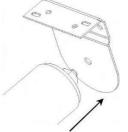
With the idle pin end in place, insert the control end into the opposite bracket. Ensure that the blind has clicked into place using the centre lug.
