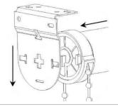
5. There is an integrated child safety device supplied with your new roller blind. This is in the form of a 'break-away' chain connector. It has been designed and rigorously tested to break free under 6kg of pressure.
